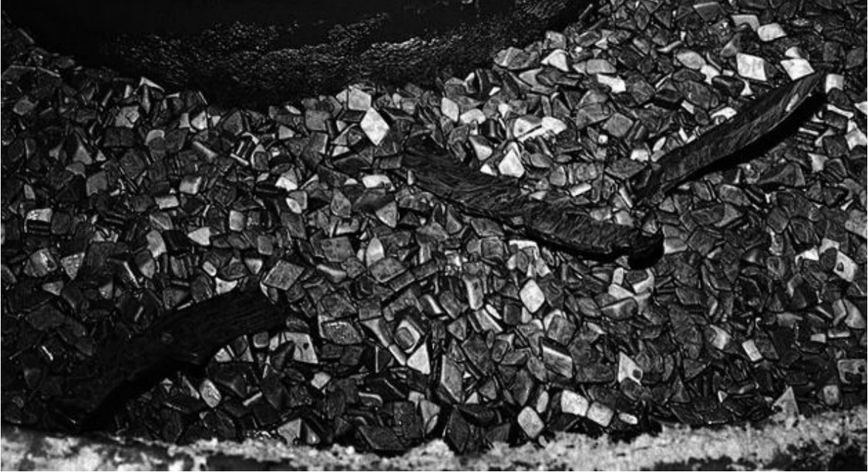
Sword blades that are polished by vibration between stones.
